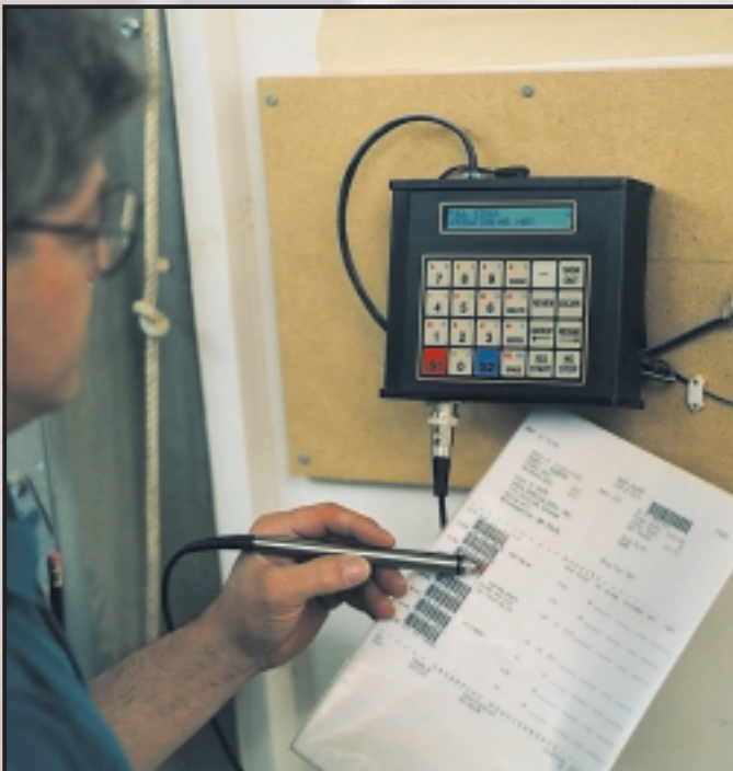
An employee can easily enter data with the keypad or the optional bar code wand.
